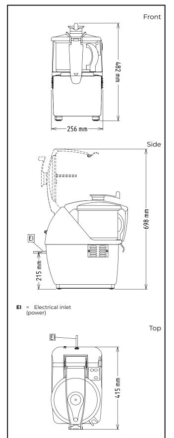
Electric Supply voltage: 200-240 V/1N ph/50/60 Hz Electrical power, max: 1 kW **Total Watts:** 1 kW Capacity: Performance (up to): 2 kg/Cycle Capacity: 4.5 litres Key Information: External dimensions, Width: 256 mm External dimensions, 415 mm Depth: External dimensions, Height: 482 mm **Shipping weight:** 25 kg
